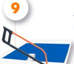
When Pancrete is hard enough, hacksaw excess PVC that was inserted in step 4. File down smooth if needed.
