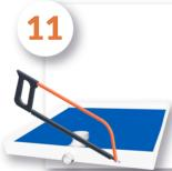
When Pancrete is hard enough, hacksaw excess PVC that was inserted in step 4. File down smooth if needed.
