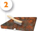
Use a wire brush or wire brush drill attachment to remove deposits and rust.
